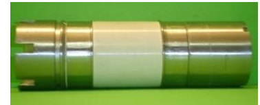
Sealing head with repaired membrane
