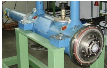
Overhaul the centrifuge bearing housing
