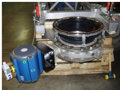
Centrifuge discharge system
