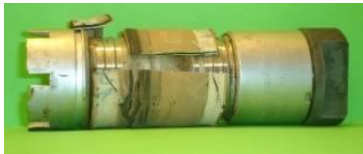
Sealing head with defective membrane
