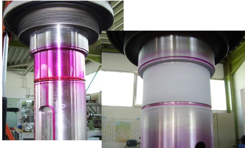
Crack detection by dye penetrant
