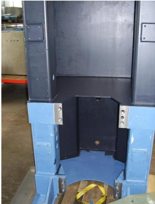
Coated with electrically conductive paint
